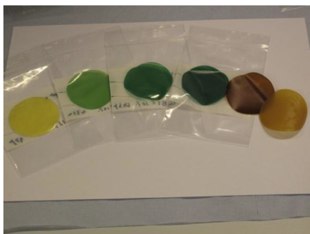
Figure 5 - Mixed matrix membranes (MMMs) containing various MOFs, used in this study. From left to right: Native P84, P84 + 10% \text{Cu}_3\text{BTC}_2 , P84 + 20% \text{Cu}_3\text{BTC}_2 , P84 + 40% \text{Cu}_3\text{BTC}_2 , P84 + 20% FeBTC and P84 + 20% MIL-53 (Al).
