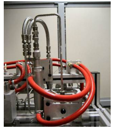
Gas permeation cell for hollow fibers, to control the temperature the cell is double walled.
