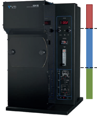
Vapor sorption equipment, SGA100, the bar indicates the 3 thermal zones.
