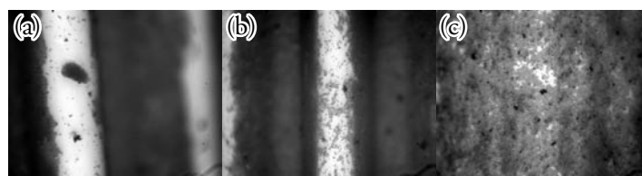
Figure 6 - Direct visual observation of the surface of hollow fibers during cross-flow yeast filtration. (a) Fin of the twisted fiber. (b) Fin of the structured fiber. (c) Round fiber.
