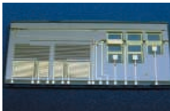
Fig.2 Realised lab-on-a-chip system for connection to a microdialysis probe. The components as indicated in figure 1 can clearly be distinguished.
