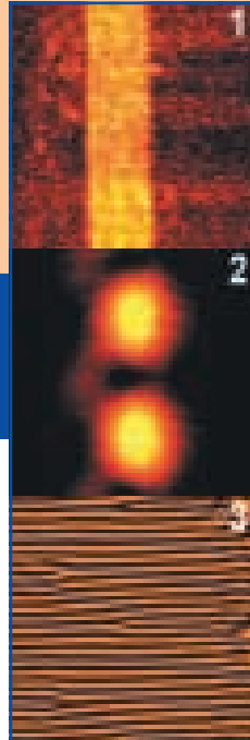
Figure 1: Measured height image of a conventional channel waveguide (all image size 10 mm x 9 mm). The ridge (height 4 nm) that confines the light is easily resolved.
