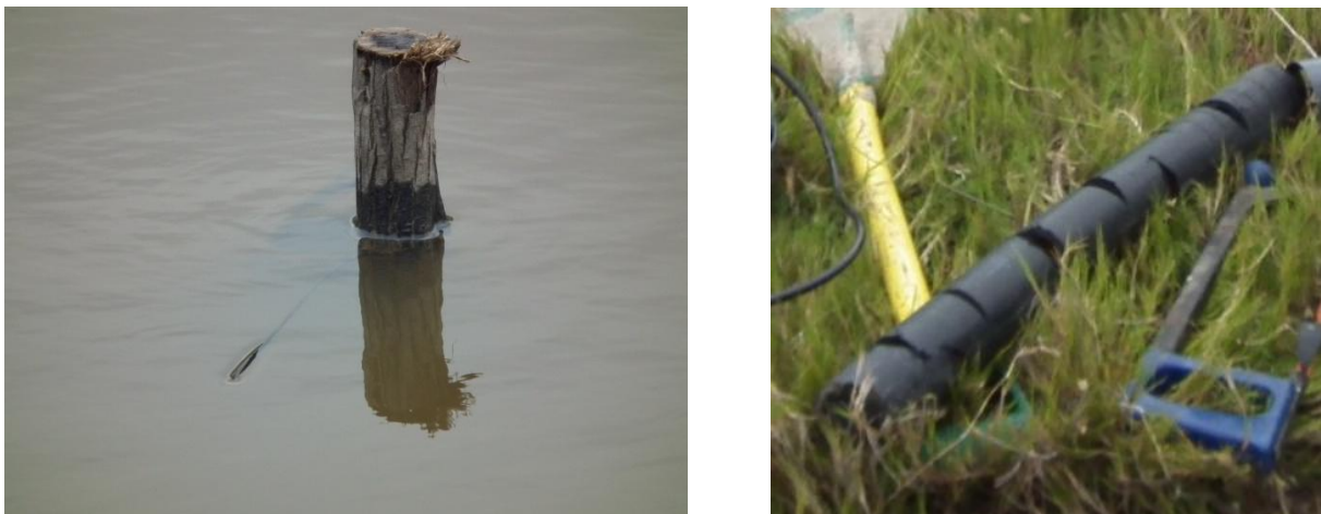
FIGURE 3.2: CTD PROTECTIVE TUBE AND SUBMERGED ATTACHMENT POLE.
