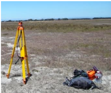
FIGURE 4.7: LEVELING INSTRUMENT SET UP.
