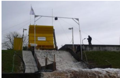
Figure 1.4. Wave overtopping simulator (Bakker, Melis, & Mom, 2013)
