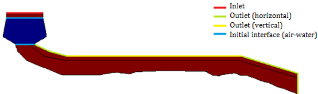
Figure 3.6. Boundary and initial conditions of the CFD simulation
