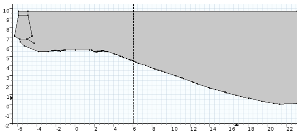
Figure 3.2. Geometry wave overtopping simulator and dike profile for the experiment in Millingen aan de Rijn
