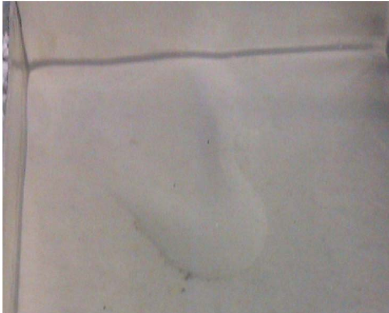
Figure 39: Photo of liquefied region after blow out
