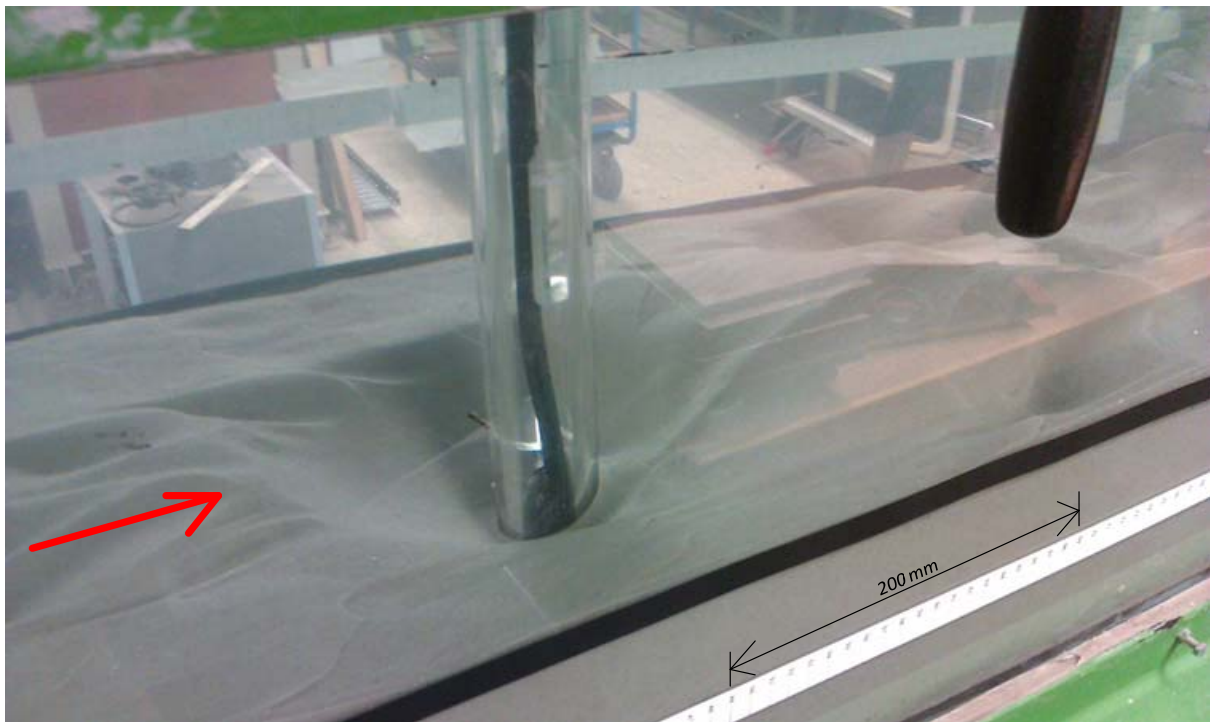
Figure 35: Scour hole after reference test.
