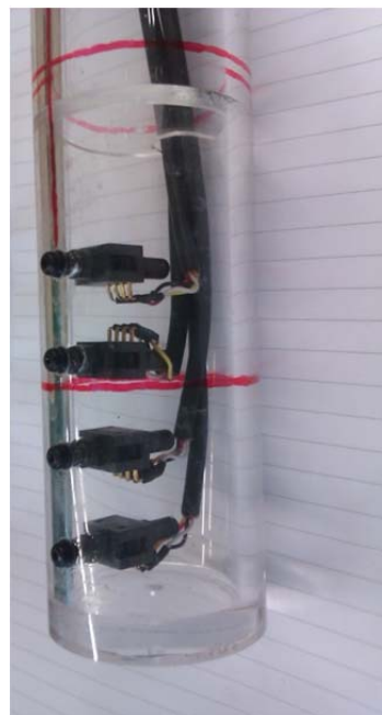
Figure A. 11: Pile with piezometers
