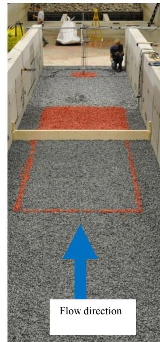
Figure 3-3: Wooden sill in front of test section 1.
