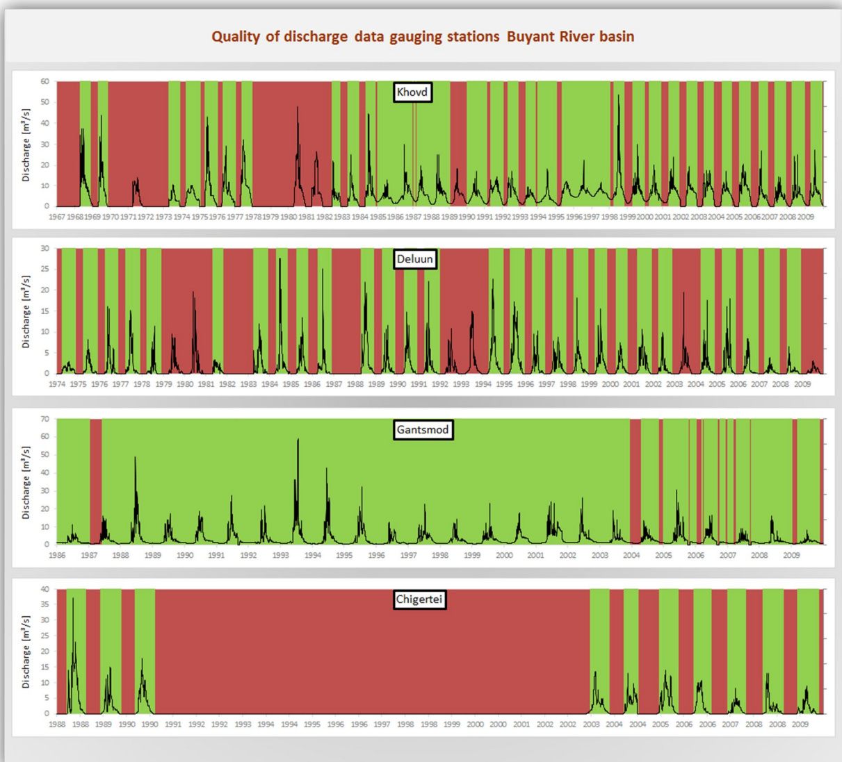
Figure 19 Daily discharge values are plotted against time for all 4 river gauging stations (IMH Mongolia). Green boxes represents reliable data, as the red boxes represents unreliable data.
