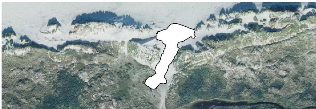
Figure 36: Overwash occurrence during the Allerheiligenstorm simulated by XBeach.
