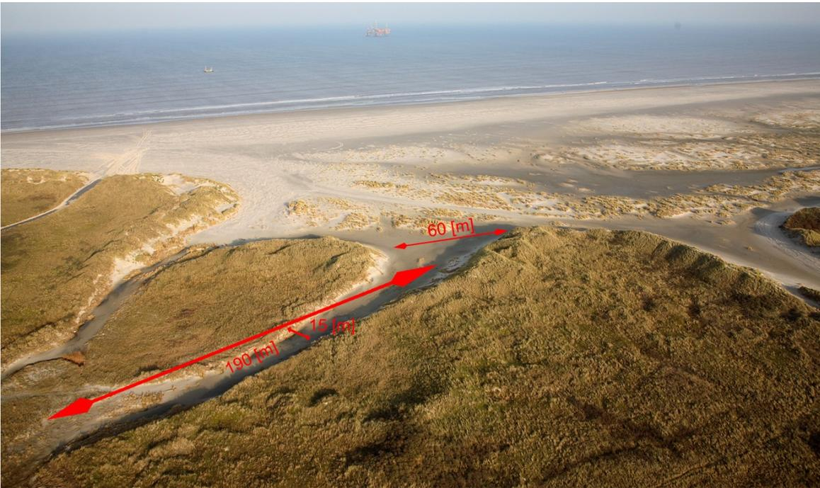
Figure 71: DeHon shortly after the Allerheiligenstorm, with the dimensions of overwash occurrence.
