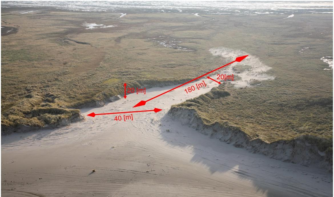
Figure 69: DeHon shortly after the Allerheiligenstorm, with the dimensions of overwash occurrence.
