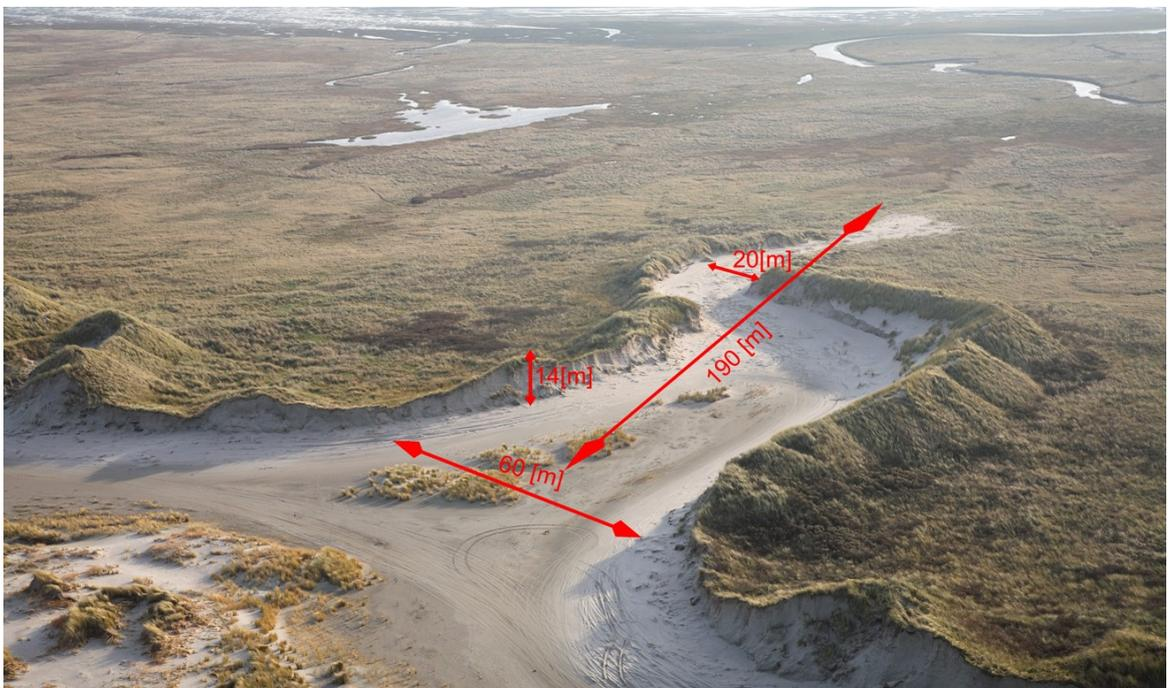
Figure 70 DeHon shortly after the Allerheiligenstorm, with the dimensions of overwash occurrence.
