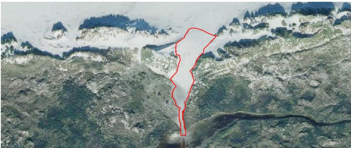
Figure 23: Observed overwash occurrence during the Allerheiligenstorm at Paal22.
