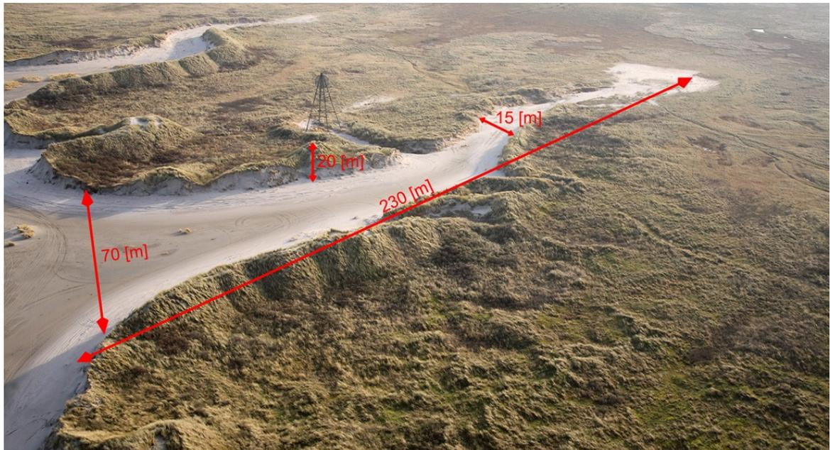
Figure 27: DeHon shortly after the Allerheiligenstorm, with dimensions of overwash occurrence.
