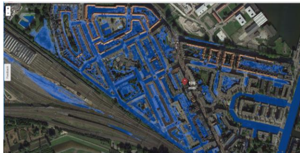
Figure 1: Screenshot of the 3Di system after a rainfall event of 100 mm during an hour for the area Houtmankade
