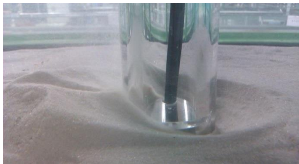
Figure 1: Initiation of scour hole formation during experiment
