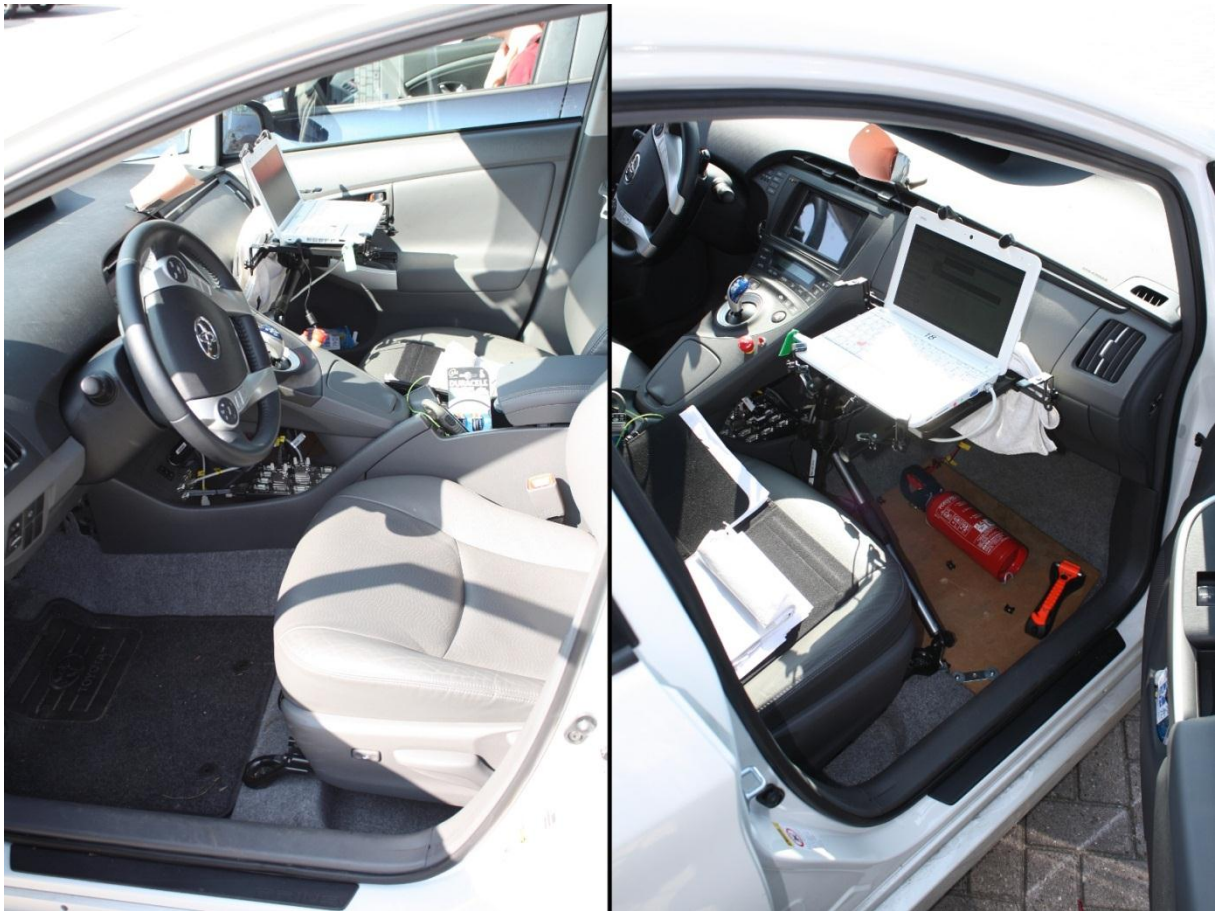
Figure 3 Interior of the instrumented vehicle: Driver's side (left) and passenger side (right). Visible on the passenger side is the laptop that recorded the radar data and the small display that shows headway to the lead vehicle (on the dashboard), with cover so the driver cannot see this.
