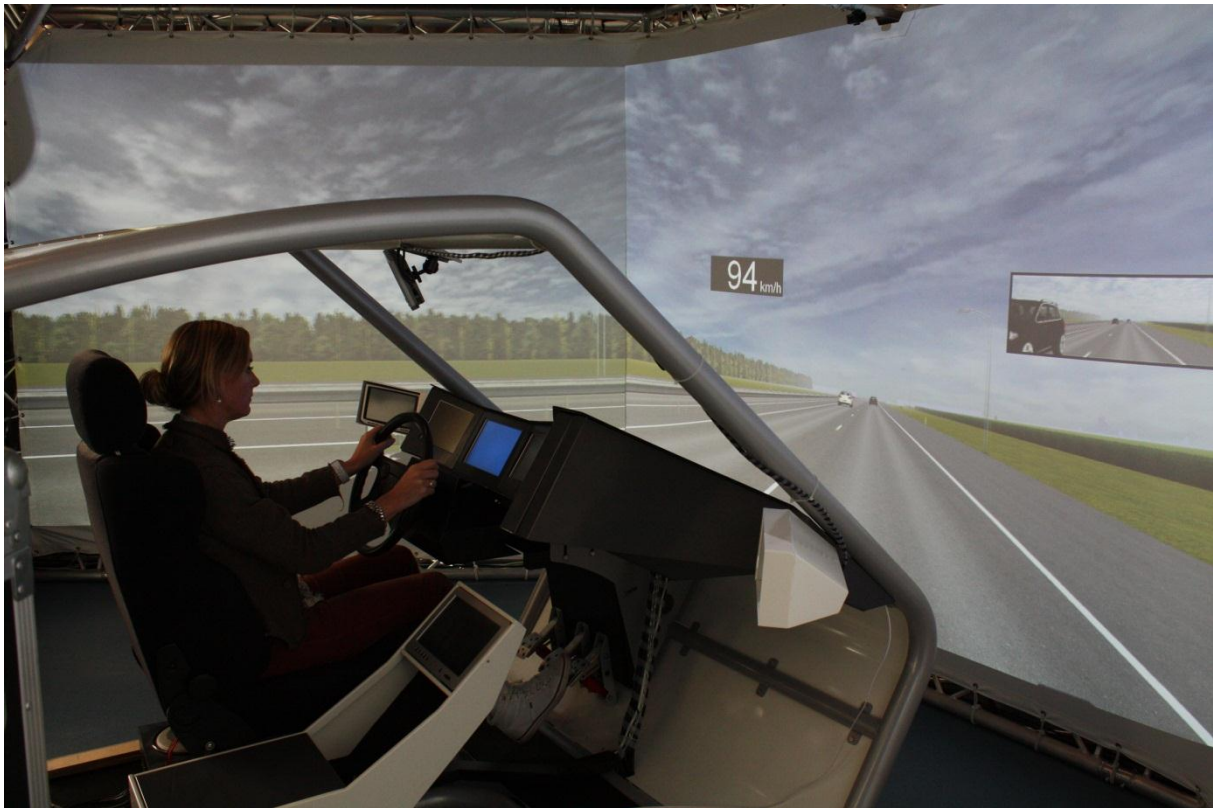
Figure 2 The UT driving simulator set-up. The operator console is behind the mock-up vehicle (to the left, out of picture).
