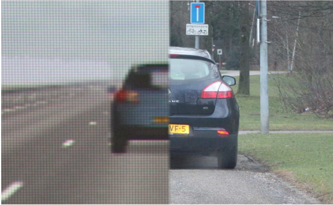
Figure 1 Apparent size of the lead vehicle at 22m from the simulator (left) and from the instrumented vehicle (right). Both photos taken from the drivers seat with the same camera, at the same zoom level.
